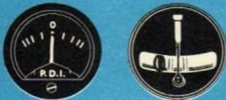
PDI CENTERED, BALL NOT CENTERED, IN STRAIGHT FLIGHT
