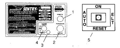
Figure 2. Pointer Model 4000-11 Emergency Locator Transmitter (ELT).
