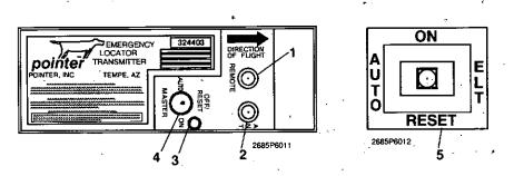
Figure 1. Pointer Model 3000-11 Emergency Locator Transmitter
