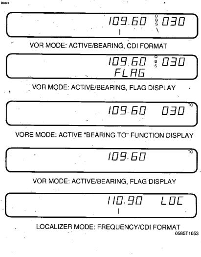
Figure 1. Bendix/King KX 165A VHF NAV/COMM (Sheet 2 of 2)
